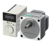
Brushless motors offer excellent energy efficiency and savings equivalent to IE4, excellent speed stability, as well as a wide speed control range. Brushless motors use permanent magnets in the rotor of three-phase motors. With Brushless motors there is no brush and commutator resulting in a maintenance free motor.
